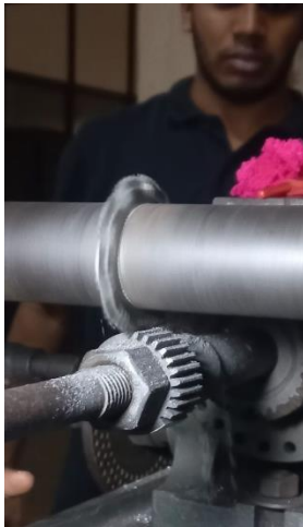
Figure 2: Cutting process of the gear
