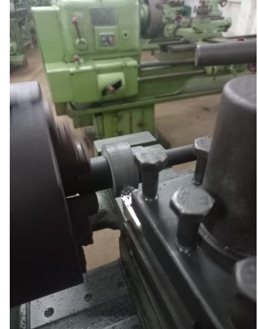
Figure 1: Turning process of the workpiece
